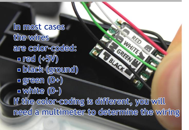
Cut the wires and solder them to the proper pads. Make sure the computer and keyboard sides are not switched.
