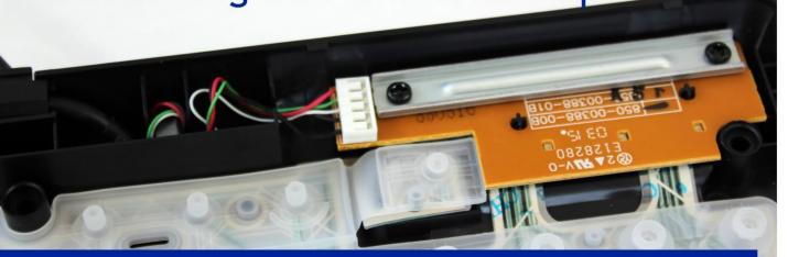
Open the USB keyboard and locate the controller inside, then find a place where the module will fit
