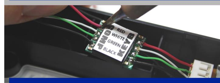
Double check the soldering, and check for short-circuits. A mistake might damage the module and keyboard.
